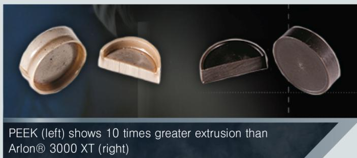
PEEK (left) shows 10 times greater extrusion than Arlon® 3000 XT (right)
